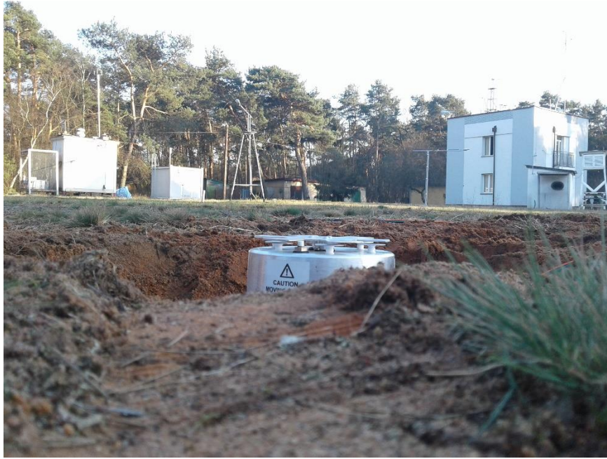
Fig. 7. 4 th Parallel Field Mill measurement at Swider, the rotating part of the head is at the ground level
