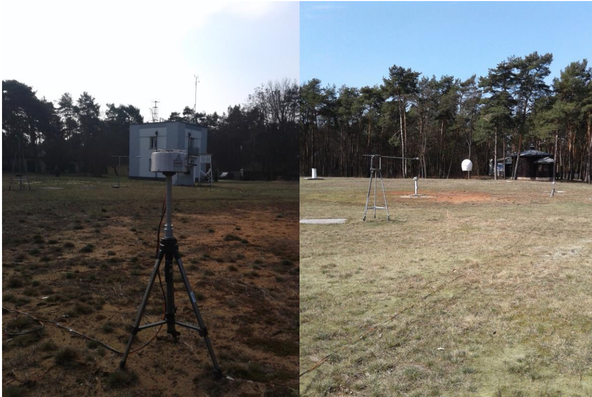
Fig. 3. 2 nd parallel Field Mill measurement at Swider, the head of the BOLTEK is at .1 m.
