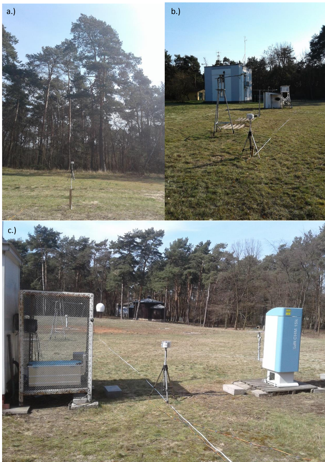
Fig. 10. The BOLTEK EFM 100 measures the E field at different points which can be affected by local circumstances (trees (a.), other Field Mill (b.) or buildings (c.))
