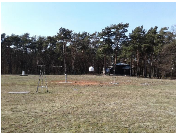
Fig. 5. 3 rd parallel Field Mill measurement at Swider, the head of the BOLTEK is at .2 m.
