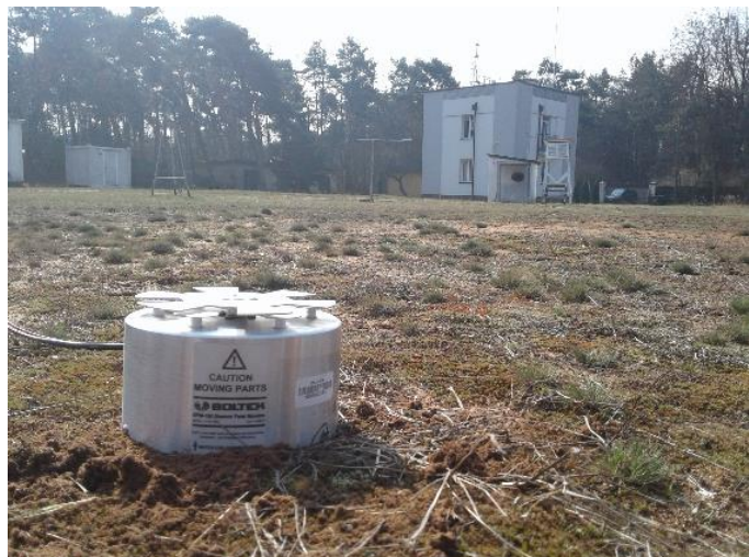
Fig. 1. 1 st parallel Field Mill measurement at Swider, the head of the BOLTEK is at the ground.
