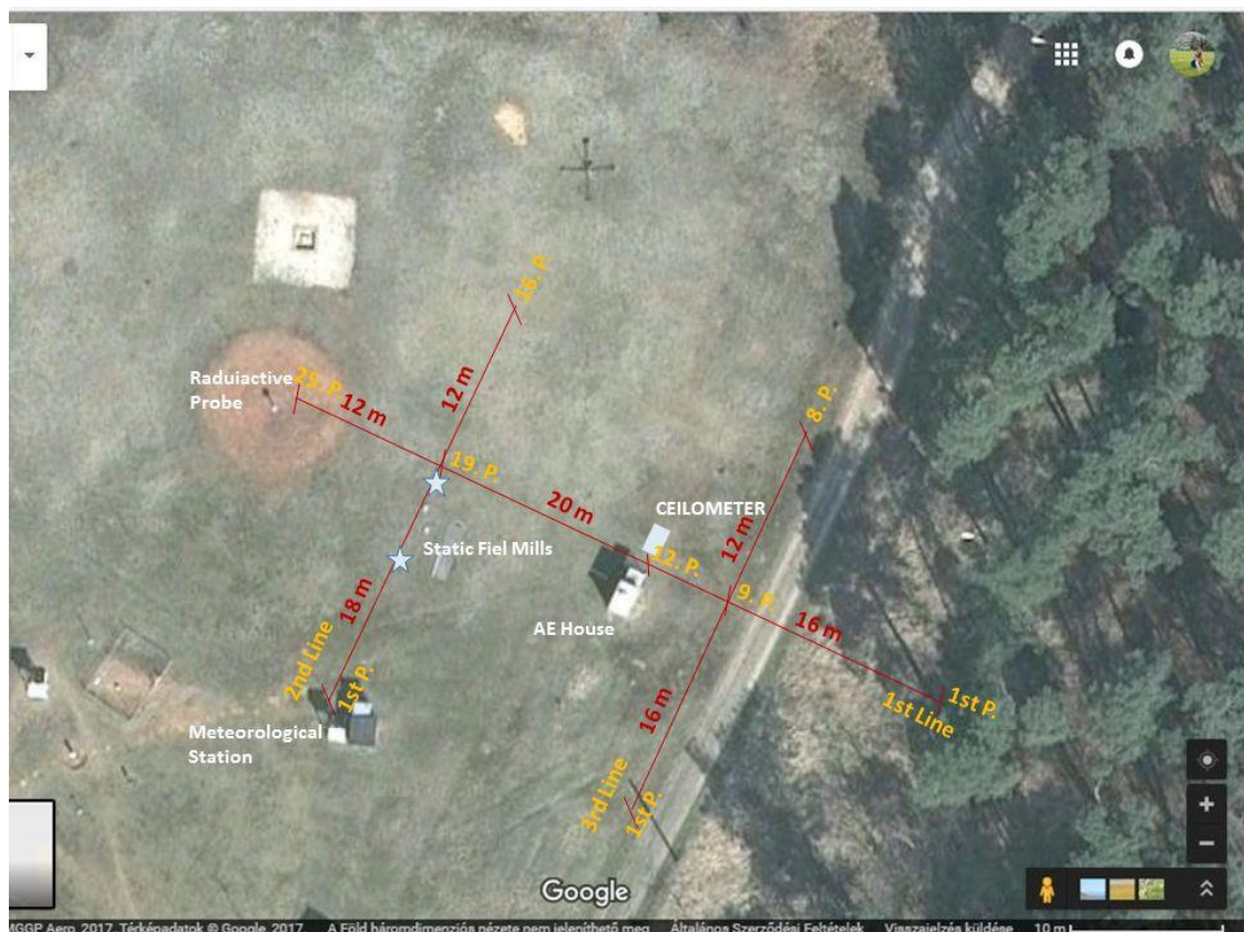
Fig. 9. The sketch of the measurement series (50 point along three lines) which has been performed at the Swider observatory. The measurement profiles are seen with red, furthermore the buildings, trees and the other instruments are seen as well.
